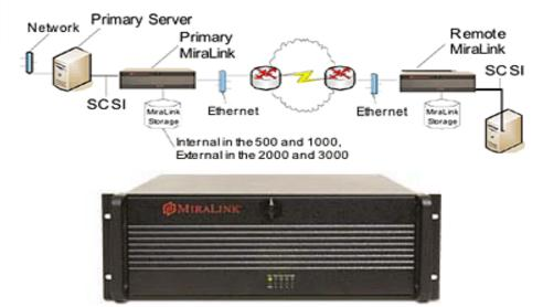
drive setup in both devices. The unit will work with almost every type of server including Windows, Linux, Novell and most of the UNIX brand of systems.
